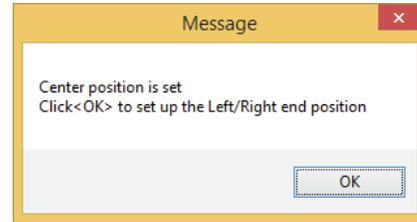
Now you will setup the left and right end points. When you have reached the desired end point click either the "LEFT" or "RIGHT" button to confirm your setting. You will be notified when each one is set. Once complete, click the OK button to exit the EPA setup.
