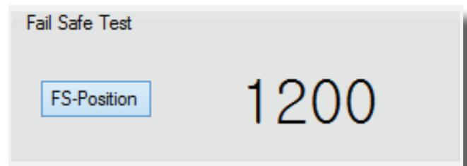
By clicking the FS-Position button, the servo will travel to its preset Fail Safe position.
