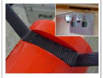
2. Install the landing gear axles with lock nut, but do not tighten yet
