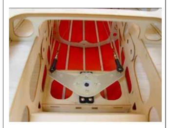
NOTICE: The coupler thread is fitted half way into ball link for further adjustment if needed to centralize rudder
