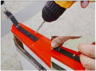
3. Install the blind nuts through the opening in the rear of the fuselage and fit screws for the tail wheel using Blue Loctite on the thread
