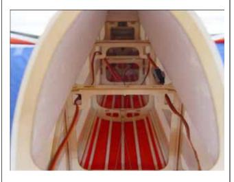
4. Cut the cover to expose the predrilled hole for mounting horizontal stabilizer to fuselage
