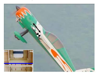
Your balance at the correct CG can be determined by positioning batteries in correct location. Mount batteries and secure with nylon ties
