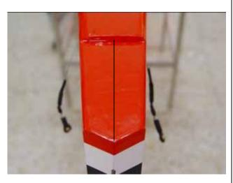
2. Drill holes on the tail wheel mounting block accordingly with the tail wheel strut taped in place or mounted with one bolt as shown
