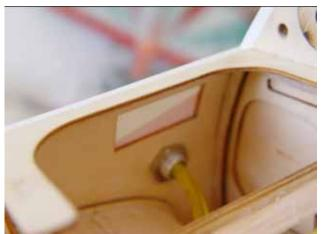
1.cut off the cover film flush with a sharp knife
