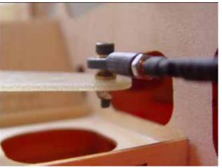
10. Turn off radio now. Reinstall the ball link, do not over tension as you may damage rudder. If tight then readjust ball link on rudder servo arms. Cables to be tensioned enough to hold rudder firm at neutral point.
