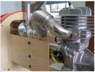
3. Use silicone coupler on exhaust joint securing with clamps as shown
