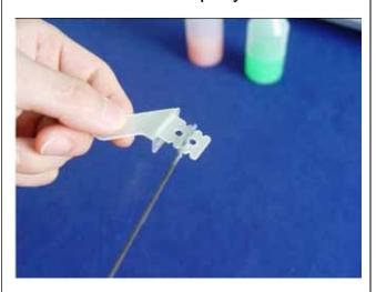
5. Slide the horns into slot slightly and Mount the locking plate in place. Align the right and left sides before epoxy has cured. Wipe away excess epoxy with rubbing alcohol
