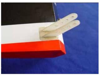
6. Make sure the horns line up (by installing the steer bolts )and align the both side before epoxy has cured
