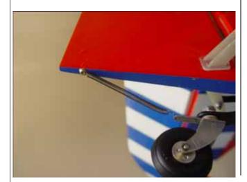
Ensure the spring has been fitted tightly for correct operation of tail wheel when rudder operates
